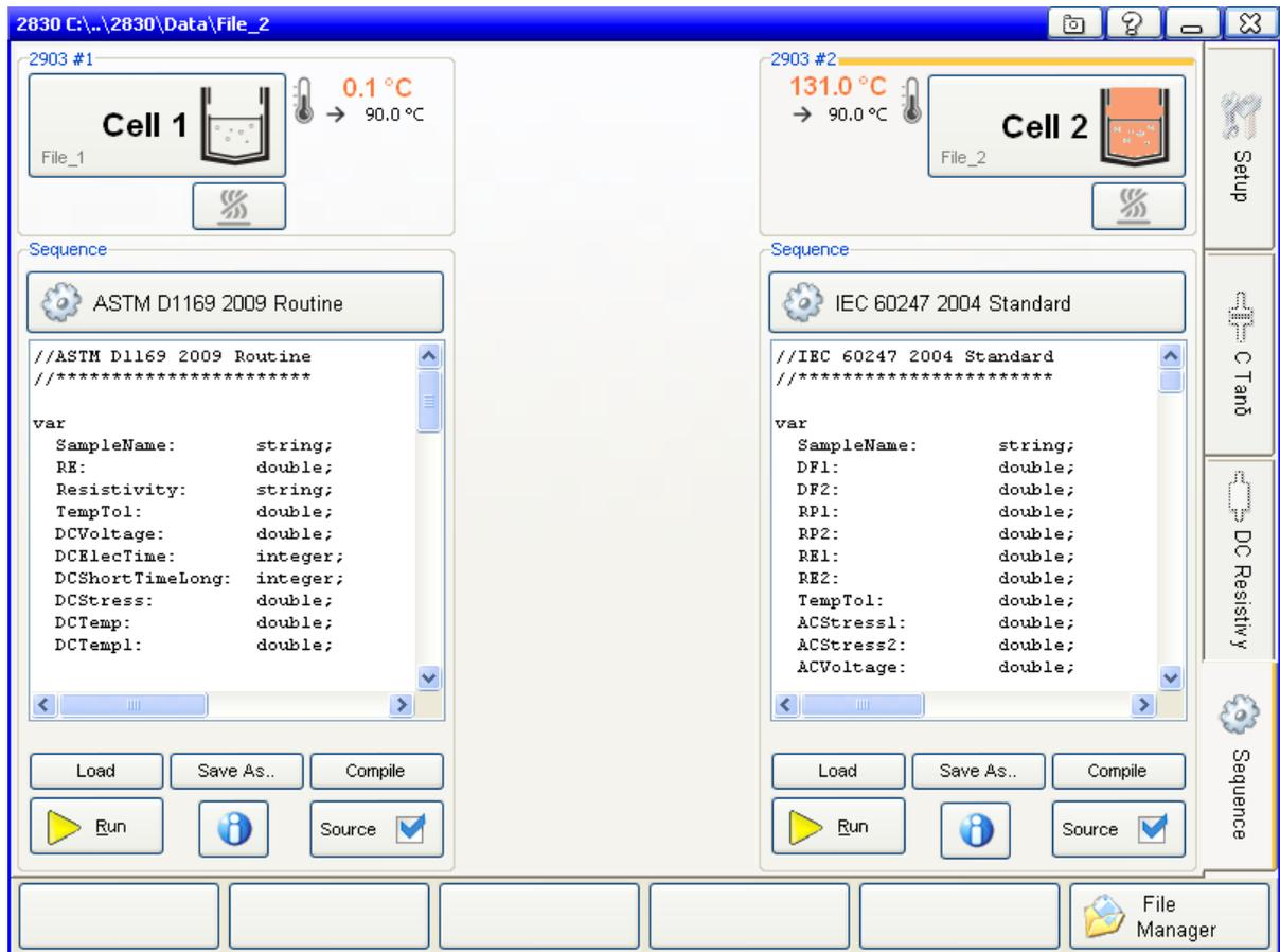
After selecting the heaters, test cells and standards both procedures can be started. (see chapter 8.7.1 Run a Sequence). To find the optimum combination of sequences and start time delay between them regarding the throughput it has to be done several tests because it depends on different factors such as cleaning and preparation time of each sample, the number of test cells that are available etc.
