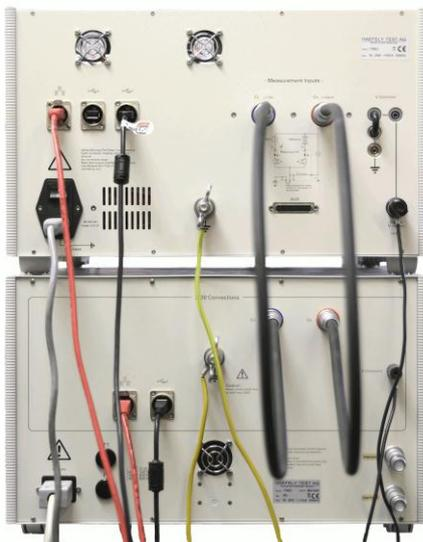
For the inter wiring of the 2830 and 2831 use only the cable which are delivered with the instrument.
