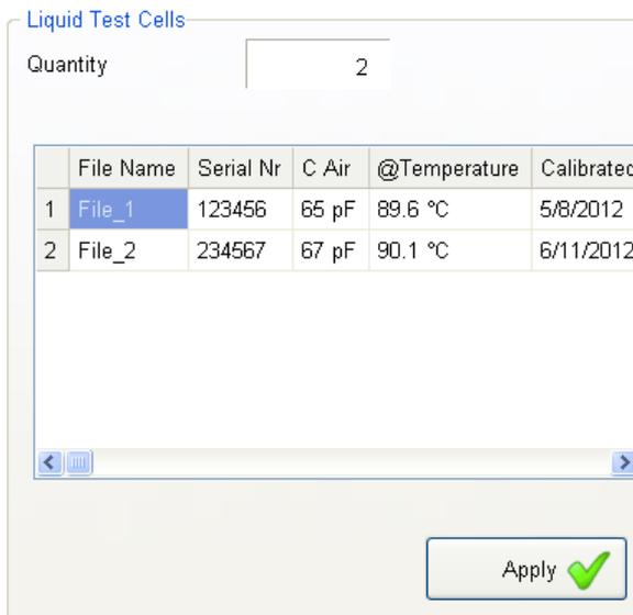
In the field “Quantity” you define how many liquid test cells you will use (the maximum are 10 liquid test cells). For all liquid test cells you have to set the “File Name” (either you make a new file or you open an existing file, see 8.3 File Manager), the “Serial No.”, the capacitance of the empty test cell (C Air), the temperature of the empty test cell, and the calibration date.
