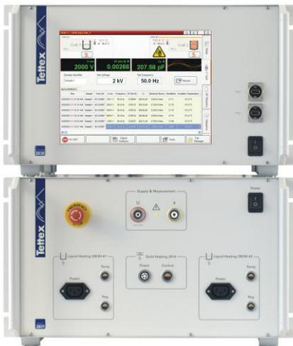
There is no special recommendation to install the oil tester. A ideal position to mount the 2830/2831 is, to put the 2831 on the table and the 2830 on top of the 2831 (see the picture on the left side).
