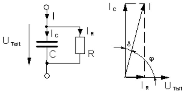
Parallel equivalent diagram of a loss capacitance with vector diagram
