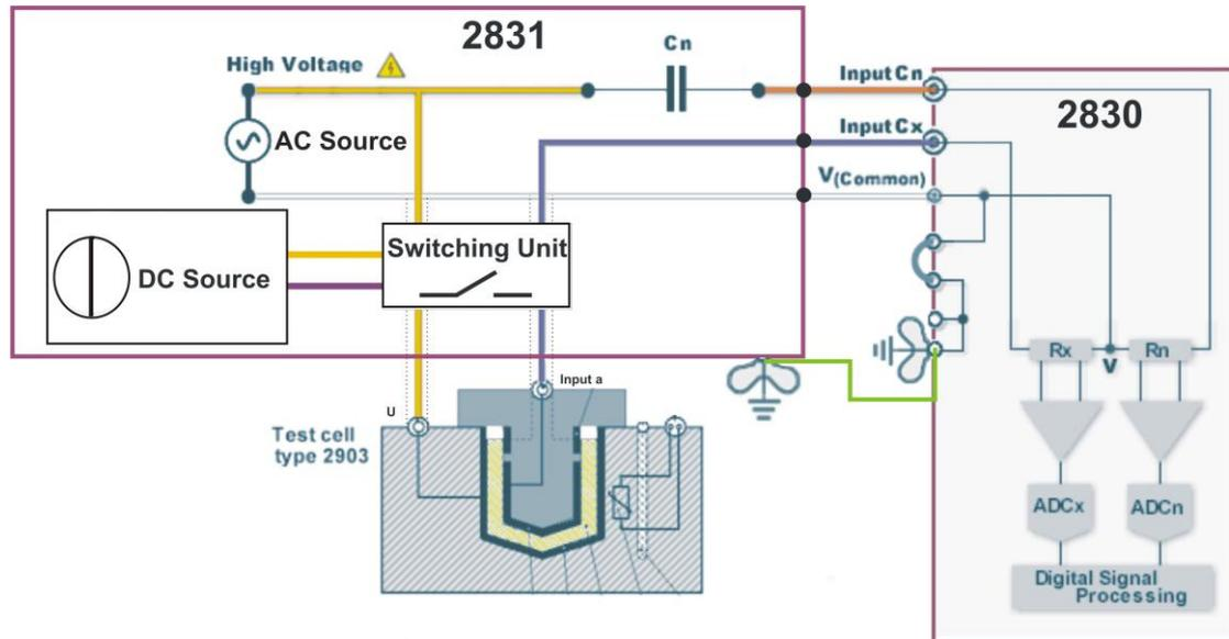
Standard connection to measure capacitance and  $\tan \delta$  of liquid or solid insulating material between high voltage "u" to low voltage "a". Connection earth to  $V(\text{Common})$  has always to be closed, else the high voltage can occurred on the  $V(\text{common})$ .
