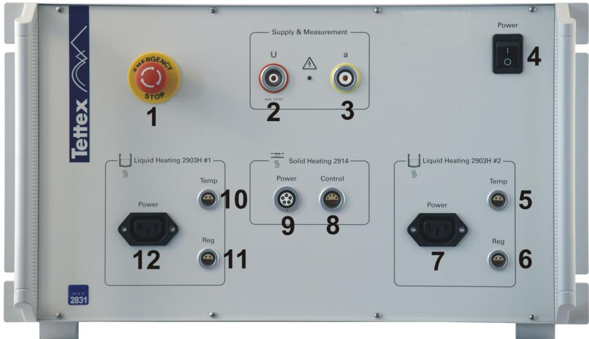
1. Emergency Switch ( Stops AC & DC power supplies and all heaters)
